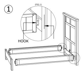
ATTACH THE RAILS TO THE HEADBOARD AND FOOTBOARD BY INSERTING THE HOOKS OF THE RAIL INTO THE SLOTS AND PUSHING DOWN THE RAIL UNTIL IT IS FIRMLY FASTENED.(FIG.1) ONCE THE RAILS ARE PLACED, FIX THEM TO THE HEADBOARD AND FOOTBOARD WITH THE SCREWS AS SHOWN IN FIG.2
